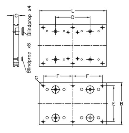
$\begin{array}{lll} B & = 185 \\ C & = 20.00 \\ d & = 298 \\ E & = 160 \\ F & = 370 \\ For bearing = 54 \\ For slide & = L/NL 76 \\ L & = 400 \\ \end{array}$
